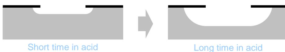
The etched surface is very smooth, similar to a polished surface (<5nm roughness).
