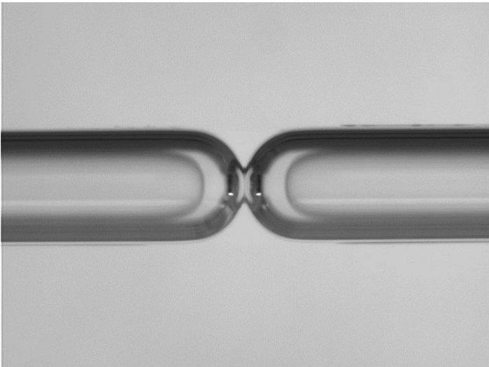
This type of constriction has several applications including the trapping of beads inside a microfluidic device.
