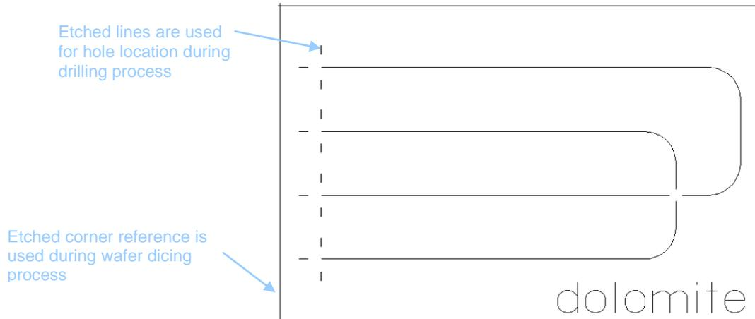
Note: For edge connection the etched corner can create a leak path on the face of the chip that mates with the edge connector. Please check all designs with Dolomite before proceeding with mask fabrication.
