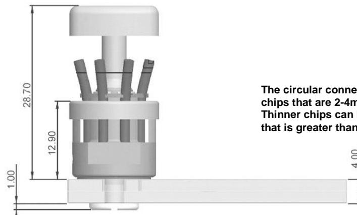
The circular connector will work with chips that are 2-4mm in thickness. Thinner chips can be used with a spacer that is greater than 12mm in diameter.
