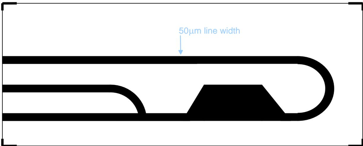
The polygons are then isotropically etched to a depth of 50µm as shown below:
