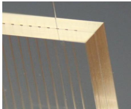
4mm thick glass microfluidic chip
