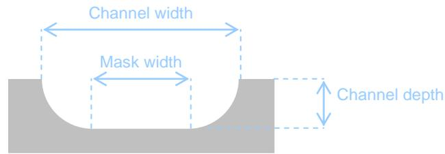
$$\text{Channel width} = \text{Mask width} + 2 \times \text{Channel depth}$$
