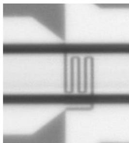
Connections to metal layers are made via holes or by taking the tracks out to the edge of the chip. Metal layers can also be deposited on the inside surface of channels as shown below:
