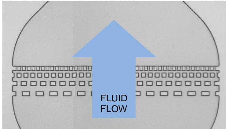
The channel depth in the image above is  $14\mu\text{m}$  and the filter has a total width of  $1500\mu\text{m}$ . The width was chosen to prevent the filter restricting the fluid flow and also to prevent it blocking up quickly.
