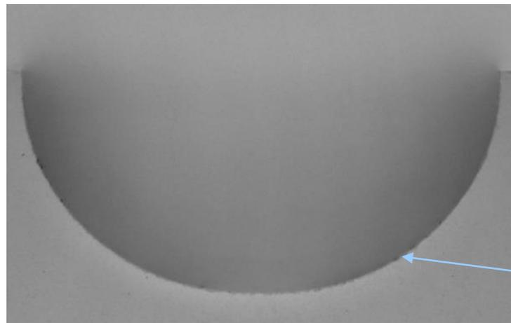
Channel etched to 250 microns depth
