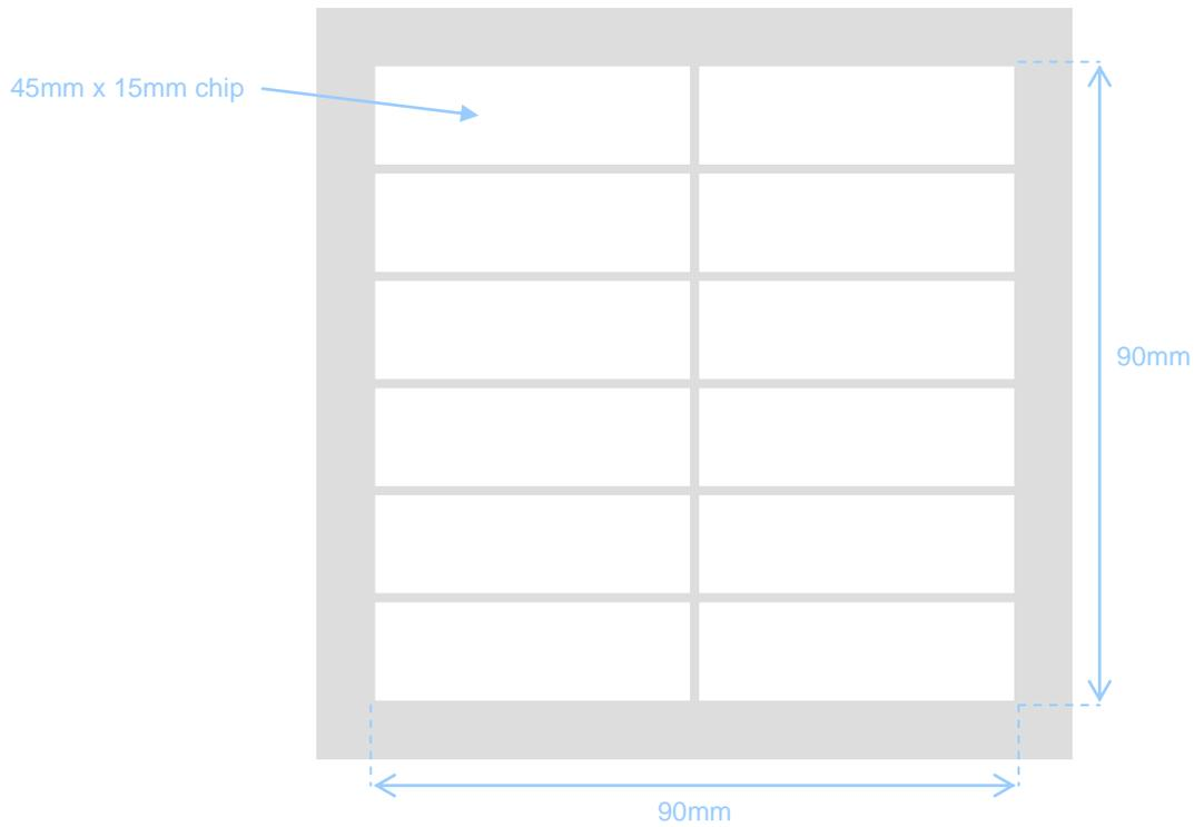
Reducing the footprint of the chips allows more devices to be fabricated from a wafer as shown below:
