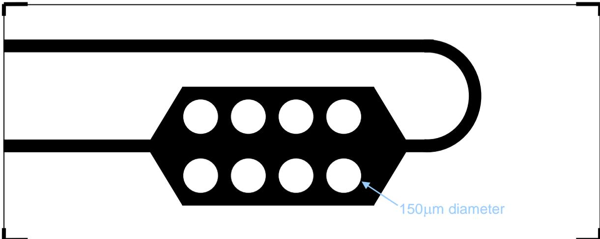
Isotropic etching to a depth 50µm results in size reduction of the raised features as shown below:
