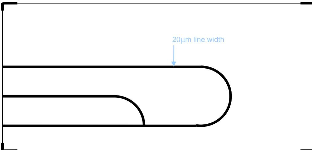
The design should include corner references for dicing (On an edge connection face they can provide a leak path so should be <0.5mm long)
