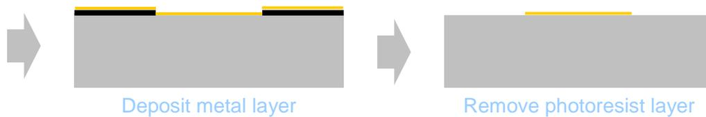
The photoresist layer is then removed and the chip is sealed using an etched top layer as shown:
