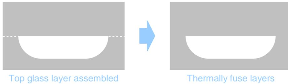
The thermal fusing process results in the two glass layers becoming one piece of glass. No adhesives or chemicals are required in this process. Once bonded glass devices can withstand pressures up to 300 Bar (standard connectors have a lower pressure rating).
