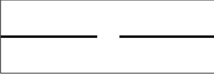
The gap needs to be  $< 2 \times$  (etch depth) to ensure that the channel will merge and produce a constriction as shown below:
