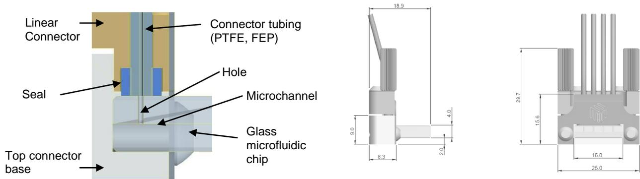
The drilled fluid holes need to be spaced 2mm from the edge of the chip as shown in the layout below:
