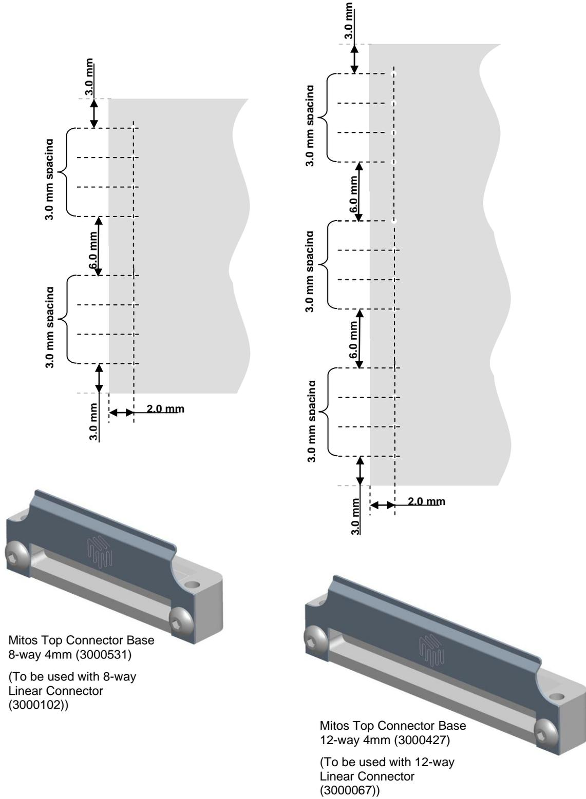
The two Top Connector Bases shown here work with chips that are 4mm thick. Custom Top Connector Bases can be supplied for thinner chips.
