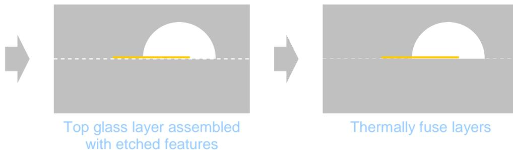
The metal layer that is deposited on the glass surface is normally between 50nm and 1  $\mu\text{m}$  in thickness. Platinum is deposited most frequently as it has excellent chemical and heat resistant properties. A wide range of metals can be deposited onto glass including gold. Adhesion of the metal layer to the glass surface is validated using a standard tape test.
