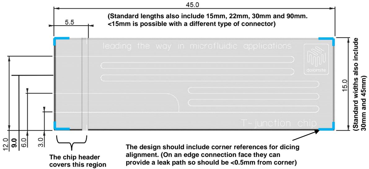
The corner references shown above in blue are required for alignment during the wafer dicing process. If you are designing the whole mask it is important to include these lines so that they are etched into the glass wafer. It is important to make sure these lines do not create a leak path on the face of the chip that will mate with an edge connector. The design team at Dolomite will be able to check this before proceeding with mask manufacture.
