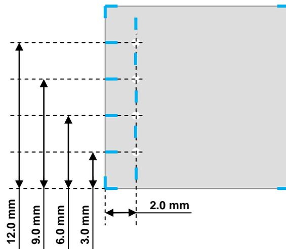
The corner references shown above in blue are required for alignment during the wafer dicing process. If you are designing the whole mask it is important to include these lines so that they are etched into the glass wafer. It may also be necessary to include additional references for hole drilling as shown above. The design team at Dolomite will be able to check this before proceeding with mask manufacture.
