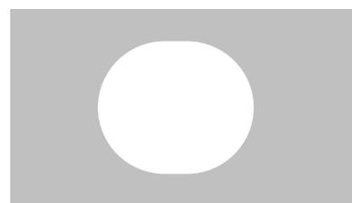
Near circular channels can be formed with a narrow mask line
