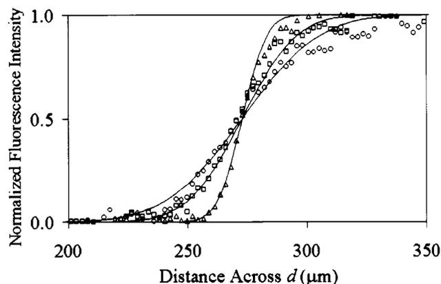
Figure 6. Fluorescence intensity profiles for the distribution of AB580 (with no HSA) across the  $d$  dimension at a distance of 5000  $\mu\text{m}$  downstream. Flow rates are 83.3 ( $\circ$ ), 416 ( $\square$ ), and 833 nL/s ( $\triangle$ ). Solid lines representing the free diffusion of AB580 are analytical fits using  $D = 4.55 \times 10^{-7} \text{ cm}^2/\text{s}$ .
