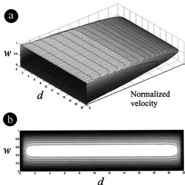
Figure 2. Normalized velocity profile in a microfluidic rectangular duct with aspect ratio ( $d/w$ ) of 22. The shape of the velocity profile (a) is uniform across the  $d$  dimension except near the walls and is parabolic across the  $w$  dimension. A contour plot of the velocity in the device cross section (b) demonstrates zero velocity at the walls (black) and uniform maximal velocity in the center (white). Solutions were obtained using a finite element analysis.
