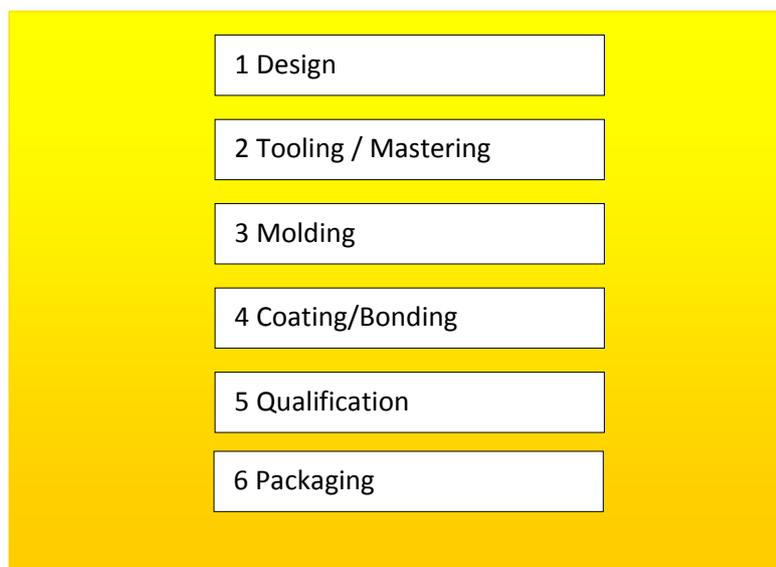
In the design phase the concept of the fluidic network has to be transformed into a component design (CAD drawing, 3D model using e.g. SolidWorks) taking into account all requirements and conditions of the molding process. At the end of this phase a complete geometrical and functional description of all needed components is generated. At this stage all mechanical tolerances and material properties should be
